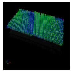
RAY CLOUD visualization, inside PIX4D software of each image. The angles represent the angle the image was captured at.
