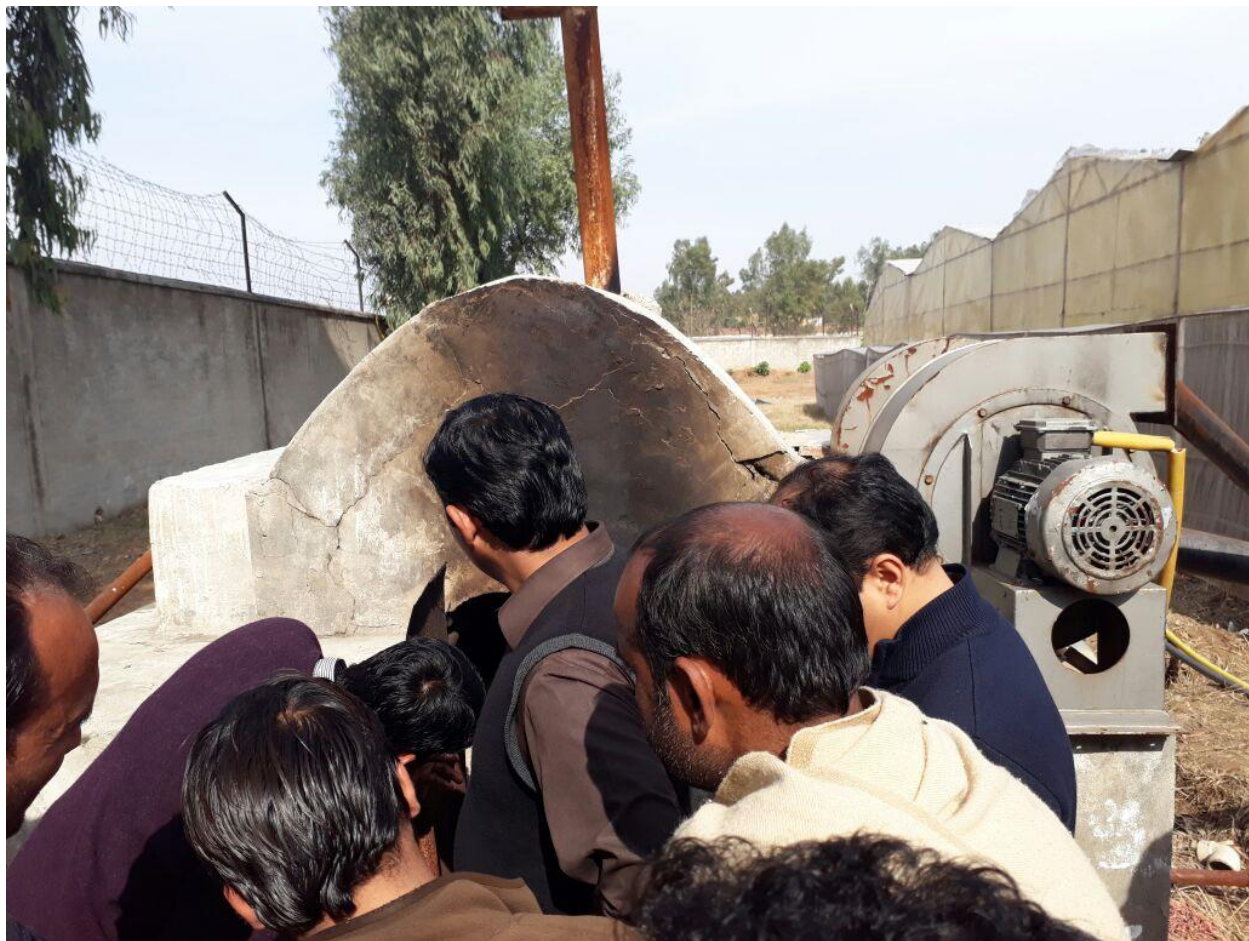
Heating system for indigenous hydroponic unit, it uses the university solid waste for heating the unit.
